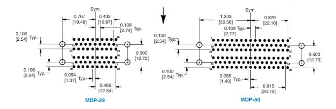
Suggest 0.039  $\pm$ 0.002 [1.00] Ø hole for contact termination positions. Suggest 0.123  $\pm$ 0.003 [3.12] Ø hole for mounting connector with push-on fasteners. DIMENSIONS ARE IN INCHES [MILLIMETERS]. ALL DIMENSIONS ARE SUBJECT TO CHANGE.
