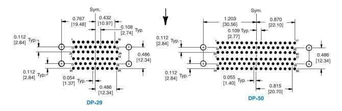
Suggest 0.045  $\pm$ 0.002 [1.14] Ø hole for contact termination positions. Suggest 0.123  $\pm$ 0.003 [3.12] Ø hole for mounting connector with push-on fasteners. Mounting holes must move 0.020  $\pm$ 0.010 [0.51] opposite direction of arrow for use of unriveted mounting bracket with connectors.
