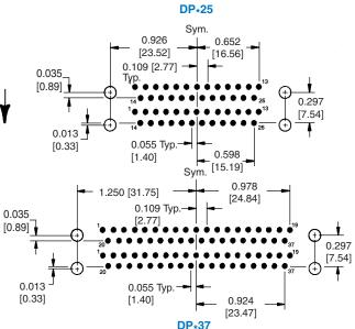
Mounting holes must move  $0.020 \pm 0.010$  [0.51] opposite direction of arrow for use of unriveted mounting bracket with connectors.
